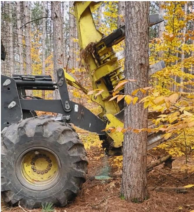
*Logging equipment adapted to spray chemicals on cut stump to prevent Heterobasidion Root Disease infection.*
