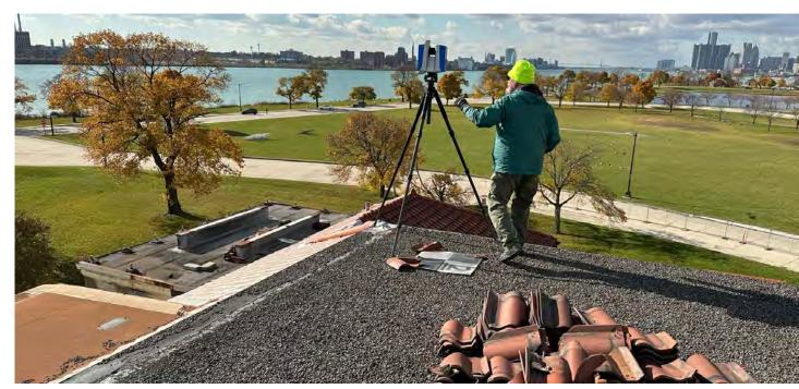
Laser scanning to measure roof dimensions between valleys..
