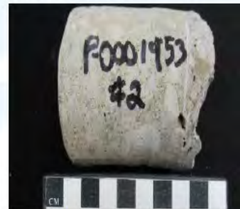
PHOTO NO. 7A: Core No. 2 – Core profile with top surface at left. A small amount of original concrete is shown at the right/bottom of the core.
