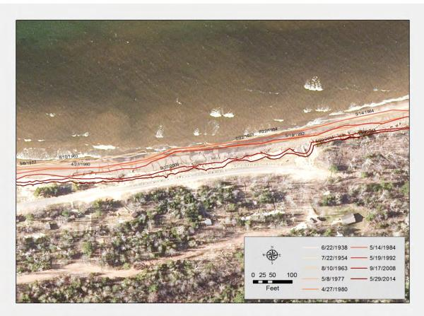
Figure 5. Bluff recession over time toward eastern end of road that serves the mini-cabins. Note relatively large change in bluff position between 1992 and 2008 bluff lines.
