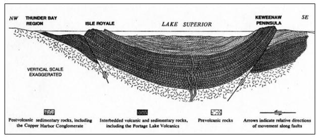
Figure 2: Cross Section of the Lake Superior Basin (USGS Bulletin 1309, Figure 38)
