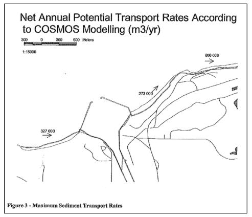
Figure 4: Maximum Longshore Sediment Transport Rates (W.F. Baird & Associates, 2001)
