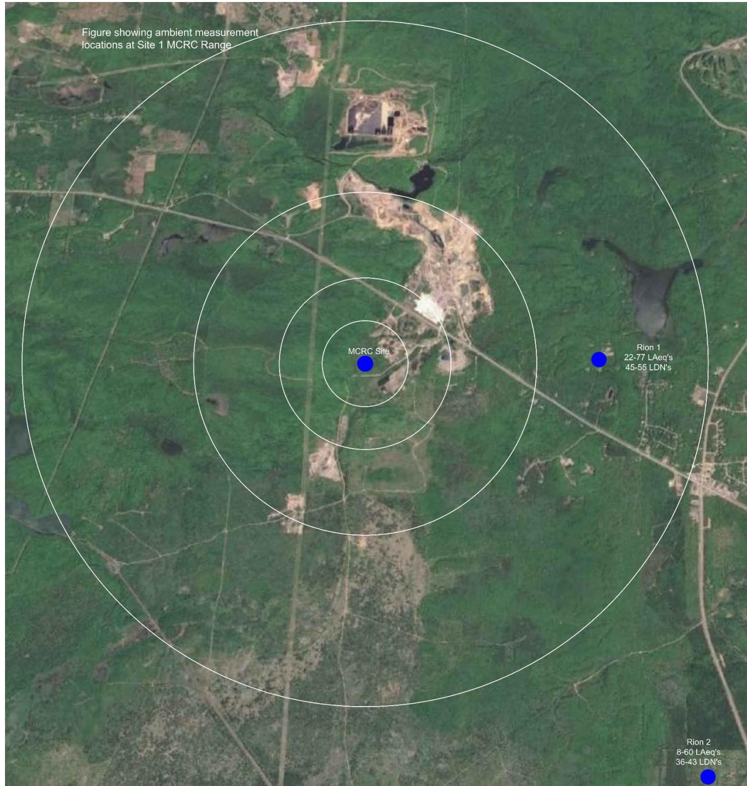
Figure A-1. Aerial photograph showing LA eq and LDN existing ambient sound levels measured at 2 locations near proposed range Site 1: MCRC.
