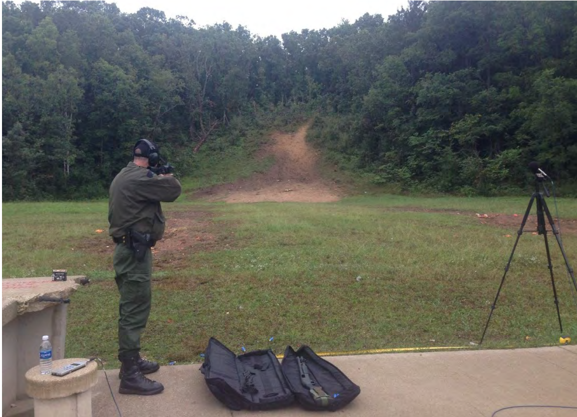
Figure 6. Conservation Officer firing at the Echo Point Shooting Range as it existed in 2016. The measurement microphone was located 10 ft. to the side of the shooter in this photograph. There are no obstacles between the shooter and the microphone. The same situation occurred when the microphone was 10 ft. in front of the shooter and 10 ft. behind the shooter in 2016. The direct sound from the gun has a clear path to the microphone. This is compared to the sound path to the microphones for the measurements made in 2021 when the range shed affected the sounds traveling from the firearm to the microphone reducing sound levels.
