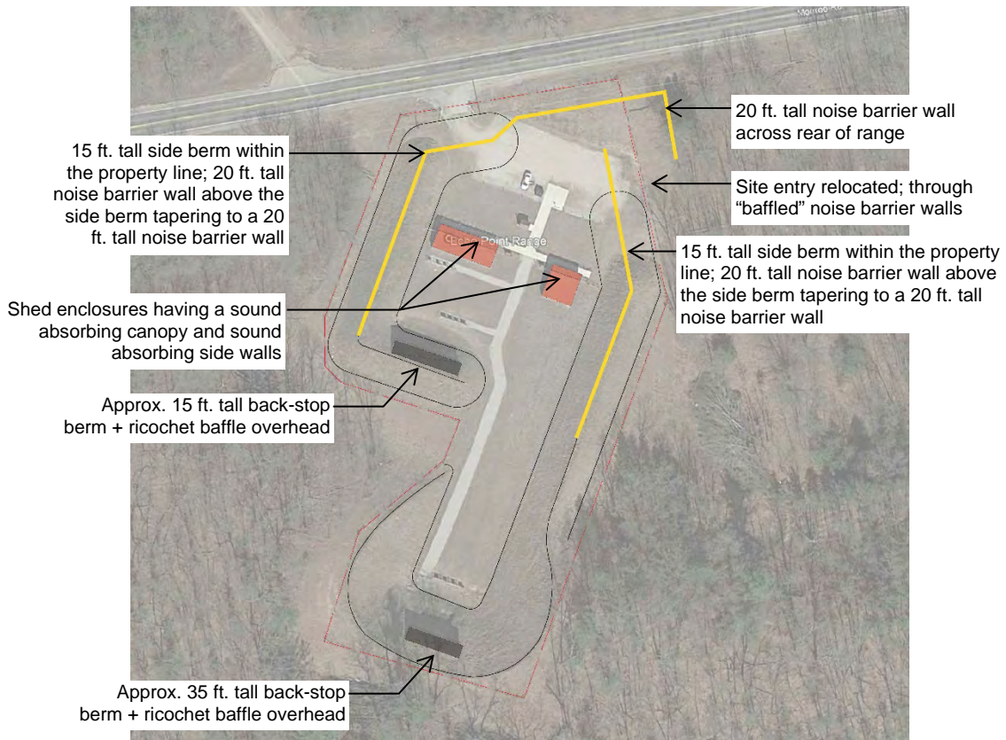
Figure 15 Concept plan diagram of the base range with the site entry relocated to the northeast corner of the site; 20 ft. tall rear walls across the range; and 20 ft. tall noise barrier walls above the side berms | Model F
