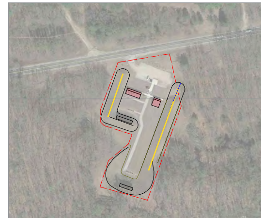
MODEL B: extend side berm east side of range; add 10' tall wall above berms
