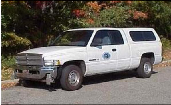
This vehicle measures the ride quality or smoothness of pavements. Operating at highway speeds, it uses a laser to measure the profile of the roadway and an accelerometer to determine the movement of the truck.
