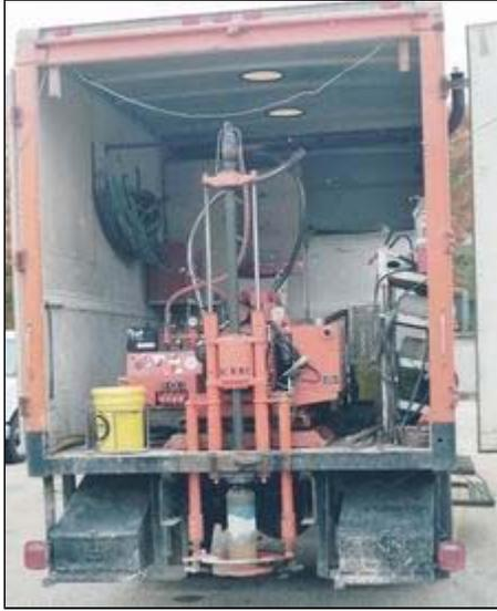
This truck is used to collect sample cores from concrete and bituminous pavement. Removing a sample from the pavement is often the best way to determine if any structural or material problems exist. The rig is also used to ensure that new pavements are built to the specified thickness.
