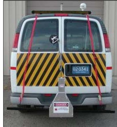
This vehicle is used to measure the underclearance of a bridge at normal highway speeds using laser technology. The system is portable and can be mounted on any vehicle with a 2 inch trailer hitch receiver. Along with the bridge under clearance data, GPS (Global Positioning System) information is recorded to mark the location of a bridge.
