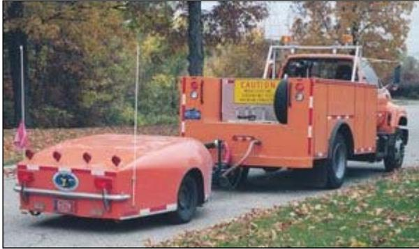
This vehicle measures pavement friction by applying water on the road and locking up the brakes on one wheel of the trailer. Horizontal and vertical forces are measured by instrumentation on the trailer axle. Once these forces are known, a friction value can be determined for the tire to pavement interface.
