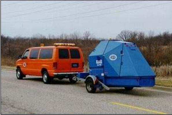
Pavements, like any other structure, deflect when loaded. The Falling Weight Deflectometer drops a weight of known magnitude on the pavement and measures the resulting deflections. From this data, the pavement's stiffness can be determined and its remaining life estimated.
