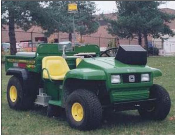
Originally developed here at Construction & Technology, lightweight profilometers are used to measure the ride quality or smoothness of recently constructed pavements. It operates similar to a full size Profilometer, but its lightweight and low tire pressure allows it to be driven on concrete pavements within a few hours of placement.
