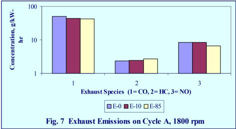
A comparison of exhaust emissions for cycle A are shown in Figures 6 and 7 for engine operation at 2400 rpm and 1800 rpm, respectively. The use of E-85 reduced NO emissions over the cycle at both the engine speeds. Not much difference was found in CO levels between the three fuels. As stated before, the mixture A/F ratio was regulated except for the inherent variations encountered in a carburetion system. Depending on the extent of these
