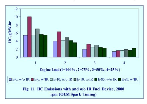
Figure 11 shows HC emissions with and without the fuel-conditioning device in the engine fuel system. The device adversely influenced HC emissions at all loads and fuels. The impact of the device is more pronounced at high loads and E-0 and E-85 fuels. The HC emissions with E-85 generally increased but the increase was lower than those realized with the E-0 and E-10 fuels.
