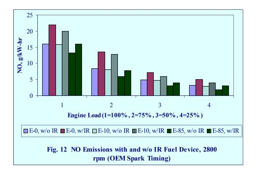
The presence of the fuel-conditioning device in the system increased NO emissions, as shown in Figure 12. Irrespective of the type of fuel the device contributed to an increase in specific NO emission. Similar differences were found at 2400 rpm.
