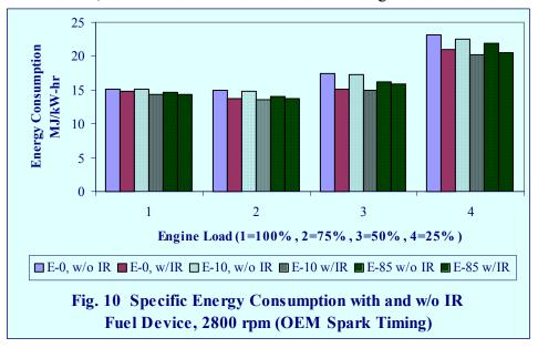
For a given load and fuel the device improved energy consumption of the engine. This pattern is evident for all three fuels and at all engine loads although the extent of improvement varied with fuel and load. Similar patterns were observed at 2400 rpm.
