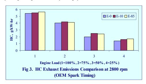
The hydrocarbon (HC) levels, in general, showed an opposite trend with the alcohol blends, as shown in Figure 3. The specific emissions of HC, in general, were higher with either E-10 or E-85 compared to E-0. Some tests, conducted at low ambient temperatures, showed a much higher increase in specific HC emissions. Ethanol and its E-10 and E-85 blends have
