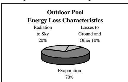
The evaporation rate from an outdoor pool varies depending on the temperature of the pool, the temperature and humidity of the air, and the wind speed at the pool surface. The higher the pool temperature and wind speed and the lower the humidity, the greater the evaporation rate.
