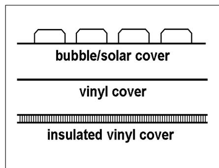
Vinyl covers are a heavier material and have a longer life expectancy. You can also get insulated vinyl covers with a thin layer of flexible insulation sandwiched between two layers of vinyl.
