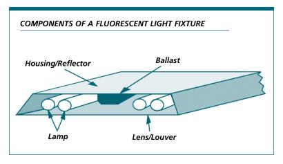
fixtures. (The number after the T represents eighths of an inch: a T-12 has a 1.5-inch diameter; a T-8, one inch). The T-8s improve energy efficiency by about 10 percent. Their electronic ballasts (devices that provide the proper voltage and current to fluorescent lamps) use 30 percent less energy than old magnetic ballasts used by T-12s.
