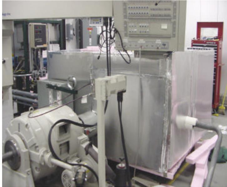
**Figure 5** Photograph of the Cold Soak Chamber ready for testing. The chamber is the large silver box shape.
