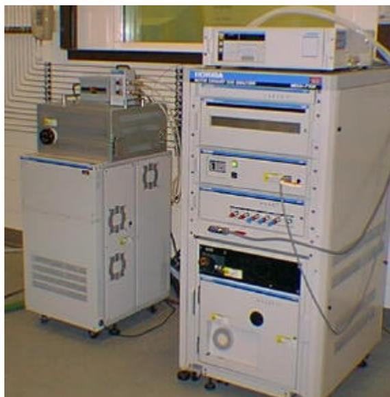
**Figure 1 Photograph of the Horiba Emissions Bench**
