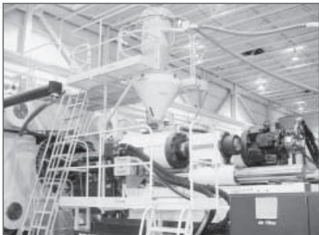
*Proper ladders and perimeter barriers are required for access to plastics injection molding machines.*
