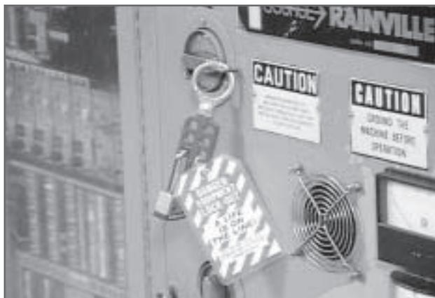
*The Lockout-Tagout standard allows an exception for minor tool changes and adjustments with the use of alternative protective measures.*
