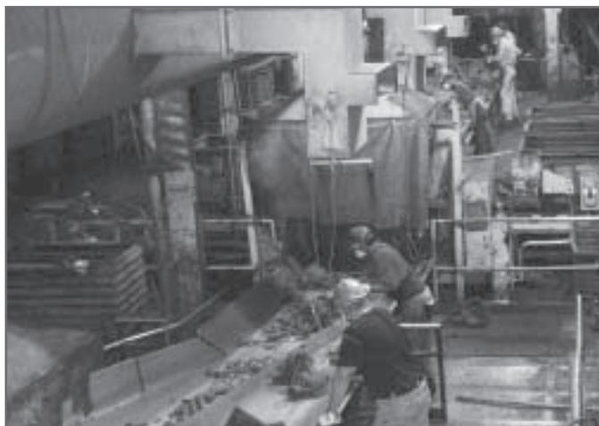
*This job requires these foundry workers to lean over a conveyor and remove defective 40-70 pound castings with a hand hook.*
