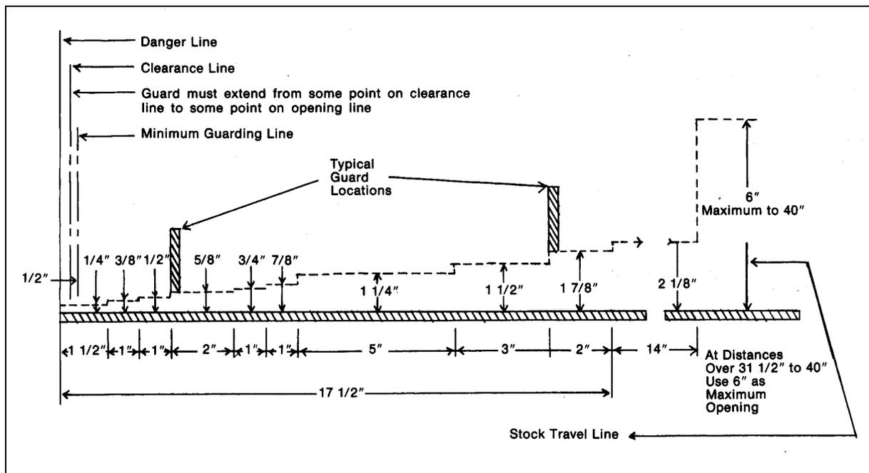
Fig. 1 shows the accepted safe openings between the bottom edge of a guard and feed table at various distances from the danger line (point of operation).
