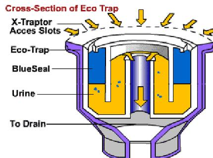
The toilet is plumbed to a standard drain line (not copper). A water supply line is not needed because this is a non-flushing urinal. In fact, there are no moving parts in the entire system. Installation costs are reduced because water lines can be costly and difficult to run to a new or remodeled part of a building.
