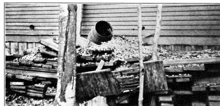
B. DRILL CORES IMPROPERLY STORED
