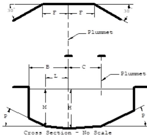
(4) "Plummet" means a vertical line which passes through the end of, and which is at the center line of, a diving board or diving platform.
