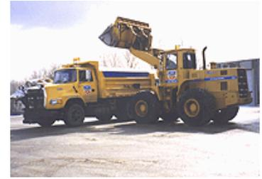
A. Loading areas must be constructed on an impervious pad and should be covered or enclosed within the storage structure to prevent the generation of salt contaminated runoff.
