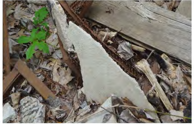
Photo 2: ACBM in demolition debris pile before removal. Photo taken on 6/29/15.
