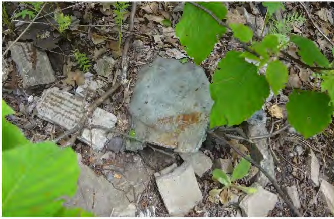
Photo 1: Asbestos containing building material (ACBM) in demolition debris pile prior to removal. Photo taken on 6/29/15.
