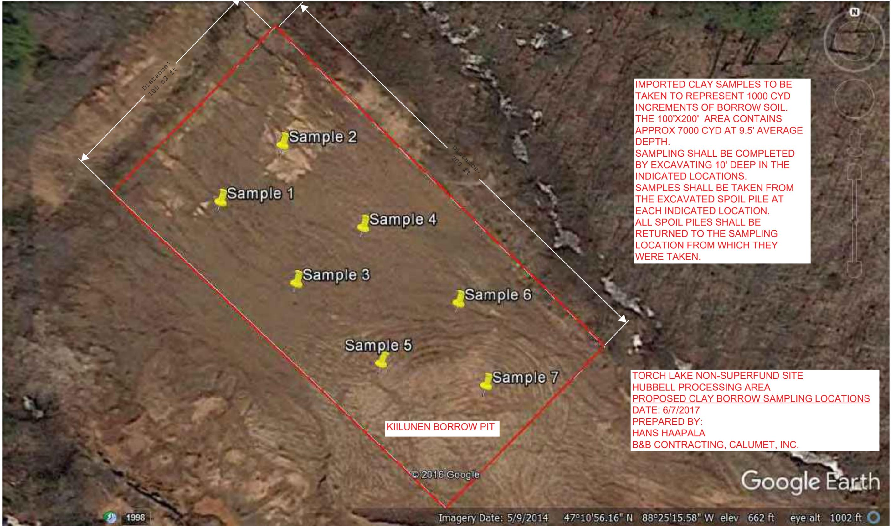
IMPORTED CLAY SAMPLES TO BE TAKEN TO REPRESENT 1000 CYD INCREMENTS OF BORROW SOIL. THE 100'X200' AREA CONTAINS APPROX 7000 CYD AT 9.5' AVERAGE DEPTH. SAMPLING SHALL BE COMPLETED BY EXCAVATING 10' DEEP IN THE INDICATED LOCATIONS. SAMPLES SHALL BE TAKEN FROM THE EXCAVATED SPOIL PILE AT EACH INDICATED LOCATION. ALL SPOIL PILES SHALL BE RETURNED TO THE SAMPLING LOCATION FROM WHICH THEY WERE TAKEN.
