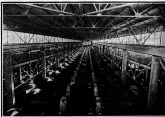
Regrinding plant, showing 64 8-ft. x 18-in. Hardinge mills
