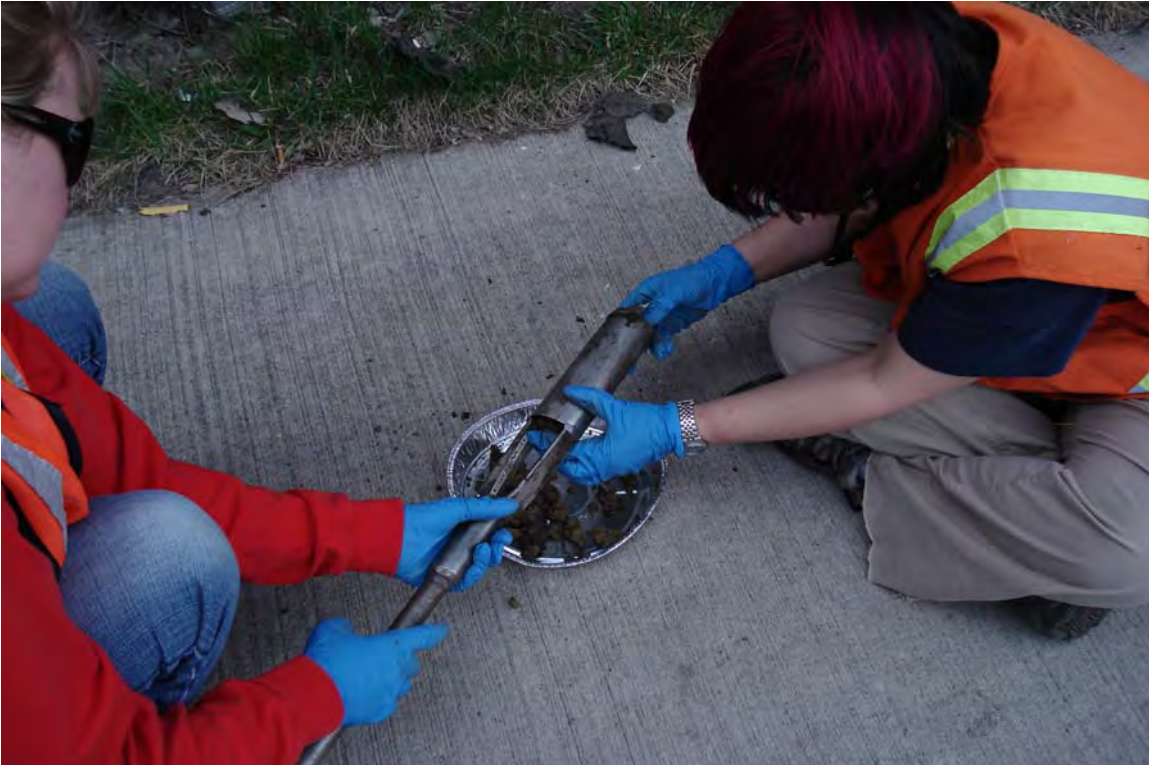
Photograph 8: 4/23/07: View of hand auger used to retrieve samples with depth.
