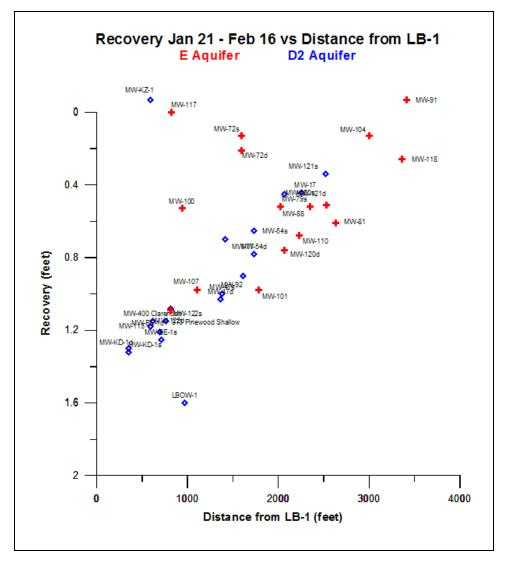
Figure 1 – Groundwater level recovery versus distance from LB-1.
