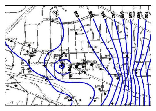
Figure 4 – DEQ contouring of May 22, 2009 data. (Does not use MW-120s, MW-121s, MW-123s, or MW-122d)
