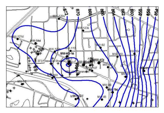
Figure 3 – DEQ contouring of May 22, 2009 data (does not use MW-120d, MW-121s, MW-123d, or MW-122d).
