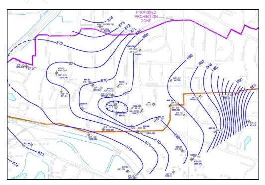
Figure 2 – Potentiometric surface measured May 22, 2009 (Taken from the PLS May22, 2009 map). This map does not use MW-54s, MW-72d, MW-120d, MW-121s, MW-123d, or MW-122d in drawing the potentiometric surface.
