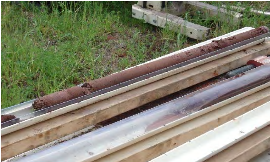
Photograph 6: 6/16/14: View looking at the soil core extracted from sample location CHLL-SB06 in the Lake Linden Recreation Area. Photograph taken by D. Liebau.
