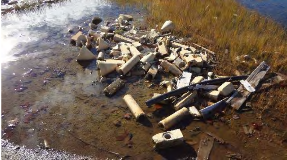
Photograph 33: 10/15/14: View looking down/southeast at a debris pile in the Hubbell Processing Area. The materials were sampled and analyzed for asbestos content. Photograph taken by D. Liebau.
