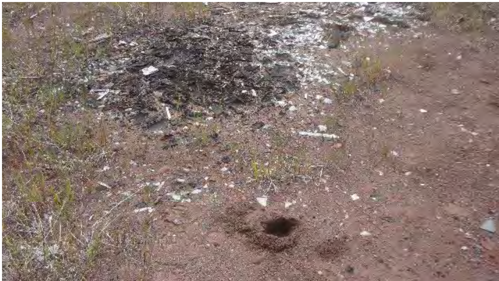
Photograph 42: 6/30/15: View looking down/southwest at surface soil sampling location SS-13 located in the Lake Linden Processing Area. The soil sample was collected to assess the presence of asbestos in soil in the vicinity of apparently burnt asphaltic roofing material and debris. Photograph taken by D. Liebau.
