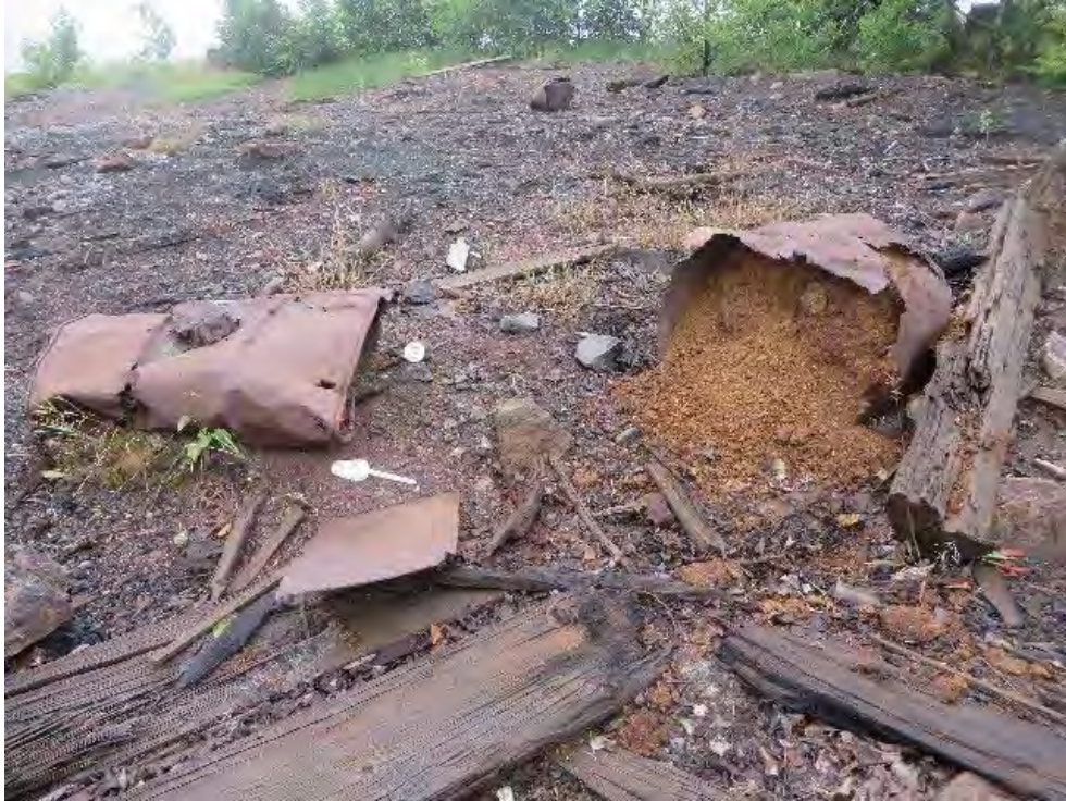
Photograph 23: 8/20/14: View looking south/southeast at deteriorated abandoned containers located in the Hubbell Processing Area. Samples were collected from the contents of each container. Photograph taken by A. Keranen.
