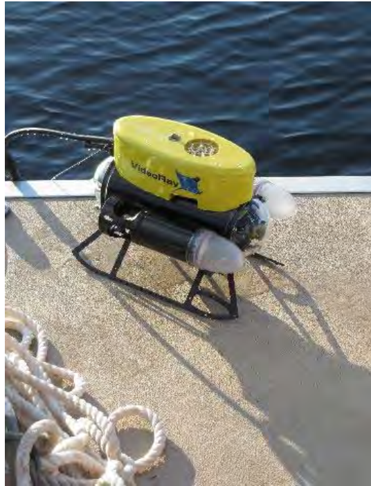
Photograph 9: 7/13/14: View looking down at the Michigan Department of Environmental Quality's (MDEQ) Geological Services Unit's (GSU) Remotely Operated Vehicle (ROV) used to visually assess underwater structures and debris. Photograph taken by A. Keranen.
