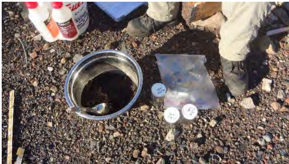
Photograph 34: 10/15/14: View looking down/north at the collection of a five-point composite sample from a debris pile located in the Hubbell Processing Area. Photograph taken by D. Liebau.
