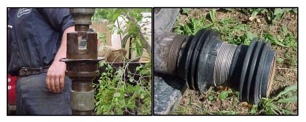
The force exerted on the formation depends on the length of the stroke and the vertical velocity of the surge block.
