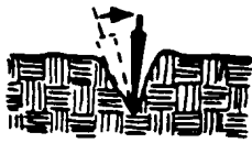
Insert bar and push forward to upright position.
