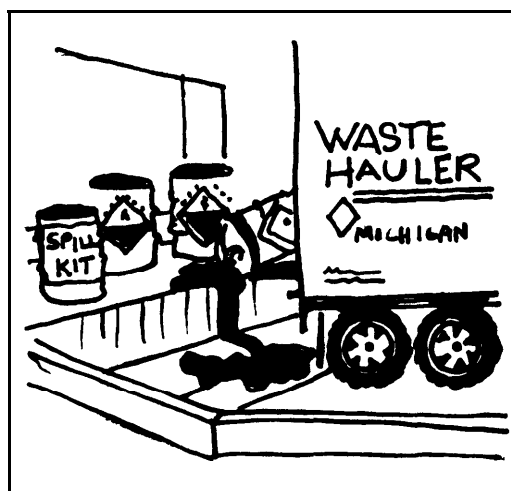
Diked loading/unloading area
