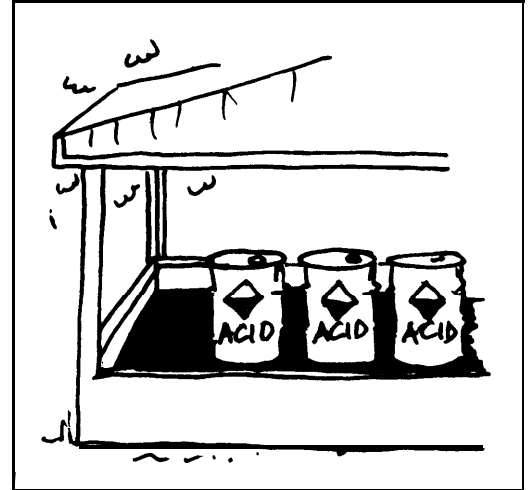
Pole shed with poured cement dike and coated floor for outdoor storage
