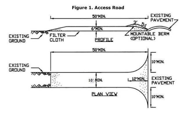
Source: New York Standards and Specifications for Erosion and Sediment Control, 2005. Stabilized Construction Entrance.
