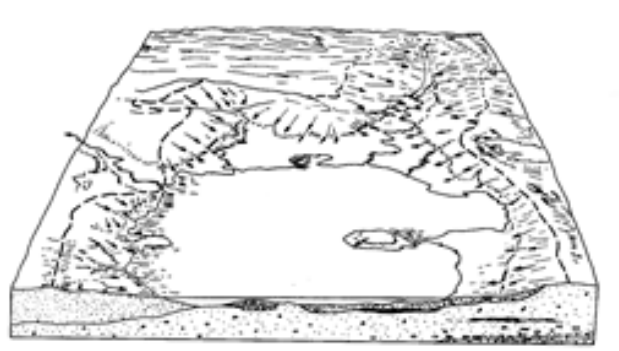
Figure 1. This diagram represents a lake and its watershed. The broken line represents the drainage divide of the watershed. The arrows depict the pattern of overland flow.
