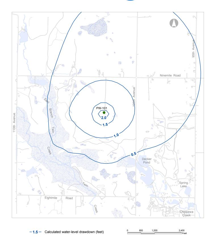
Figure A-12 Calculated Steady-State Drawdown with a Withdrawal of 150 gpm
