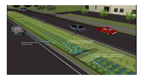
Perspective view on Green Infrastructure design for State Street reconstruction showing bioinfiltration median with runoff through curb cuts into storage cells separated by check dams. Storage is sufficient to capture more first flush road runoff.
