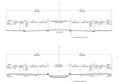
State Street reconstruction in Ann Arbor: Conventional design proposed by Washtenaw County Road Commission, with road runoff directed through curb and gutter to county drain.
