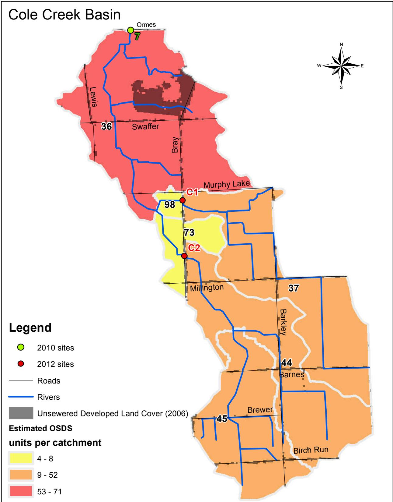
Figure F. Estimated number of OSDS units per catchment and developed land cover that is not served by sanitary sewer systems.
