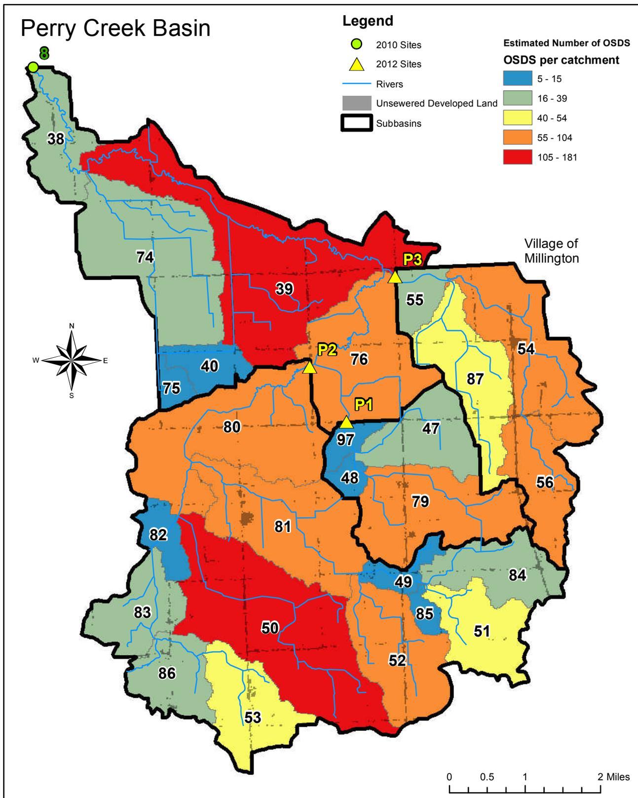
Figure F. Estimated number of OSDS units per catchment and developed land cover that is not served by sanitary sewer systems.
