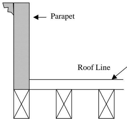
One common method of finishing the top of a load-bearing wall is to apply a large masonry cornice. While the wall may be a total of 12 inches thick, the cornice or top of the wall may be twice that size. Any such load applied to the exterior wall that is not applied in a straight vertical line with the wall to the foundation will cause stress on the wall. This stress is trying to push, pull, or twist the wall. This load is carried and
