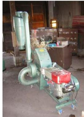
The material is ground to pass a 1/4" screen before processing into pellets. We used a small diesel operated hammer mill. The material requires no further drying and thus little additional energy for processing at this stage.
