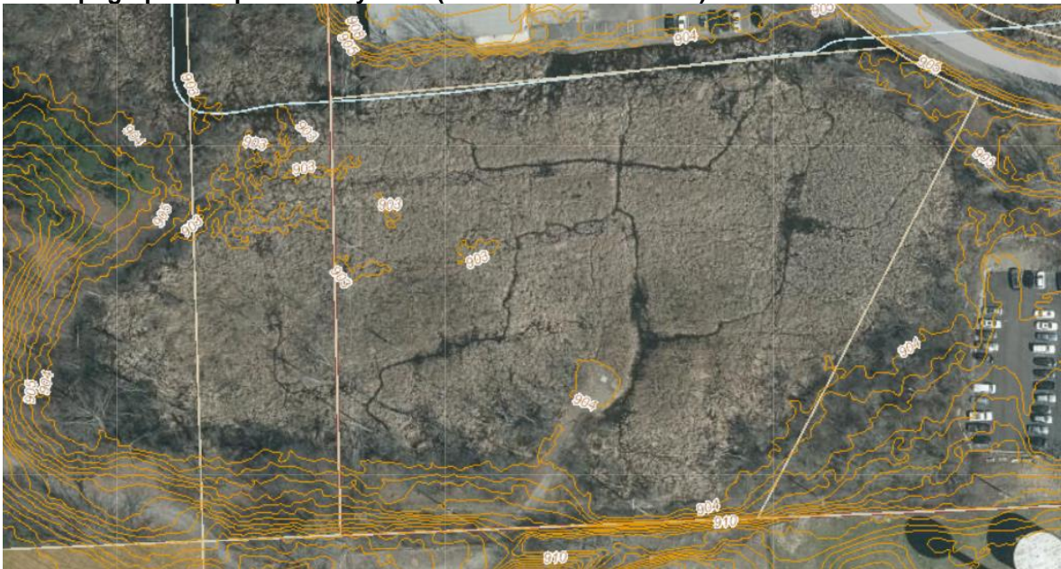
Figure 3 – Topographic Map of Marshy Area (1-foot contour interval)
