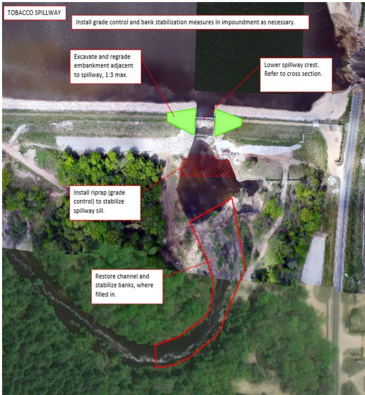
Figure 3: Proposed alternative for Tobacco River spillway.
