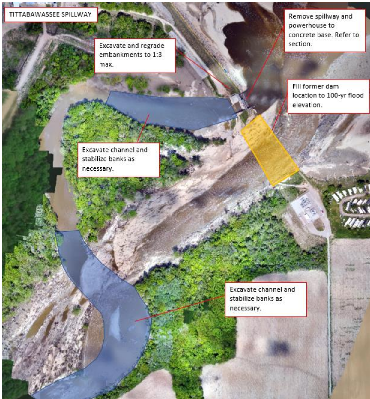
Figure 4: Proposed alternative for Tittabawassee River spillway and breach.
