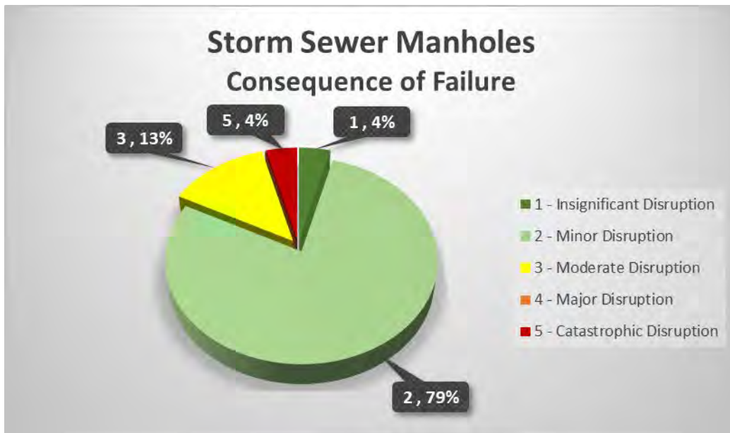
Figure 2 - Storm sewer manhole consequence of failure rating
