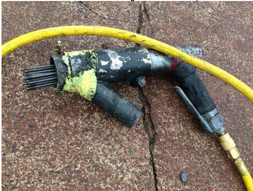
Photo 10: Pneumatic micro-chisel gun used to remove pitch mastic.
