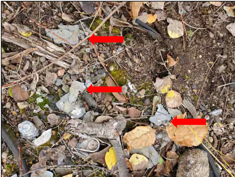
Photo 3: View of degraded pieces of black corrugated ACM (red arrows) mixed with soil at Julio Scrap yard & Tower. The black corrugated ACM and surrounding soil have been removed.
