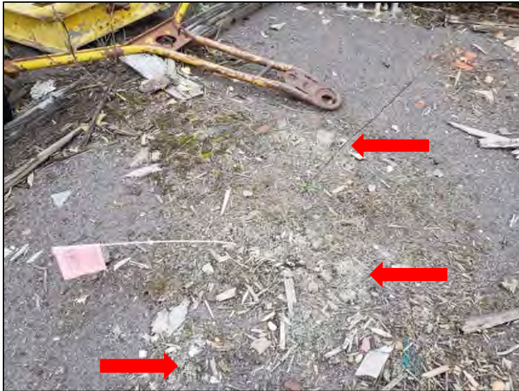
Photo 1: View of degraded TSI (red arrows) scattered on the ground adjacent to the MDNR Trail at Julio Contracting/Former Standard Oil Co which has been removed.
