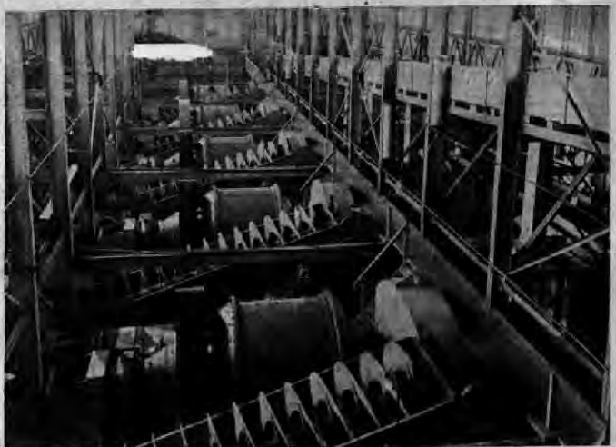
IN THE REGRINDING PLANT the sands are ground in ball mills operating in closed circuit with spiral classifiers, the overflow of which goes to flotation.
