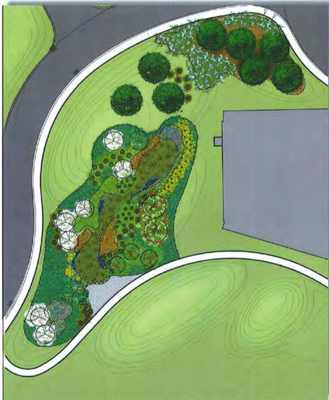
PROPOSED PLANTINGS FOR STORM WATER MANAGEMENT - EXISTING SITE BURMS TO REMAIN
