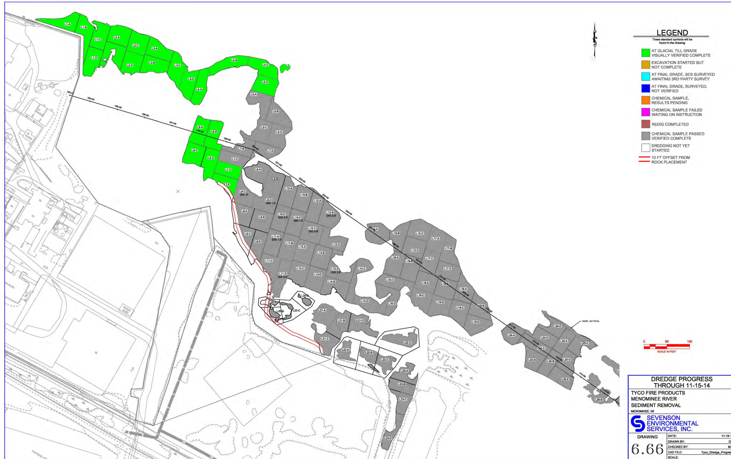
Map 3. Page 1. Ansul Arsenic Site, November 15, 2014 status of the removal of Menominee River arsenic contaminated sediment delineated by dredge management unit.
