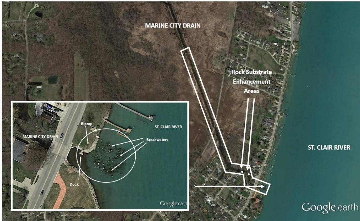
Figure 13. Location of the Marine City Drain Habitat Improvements project.
