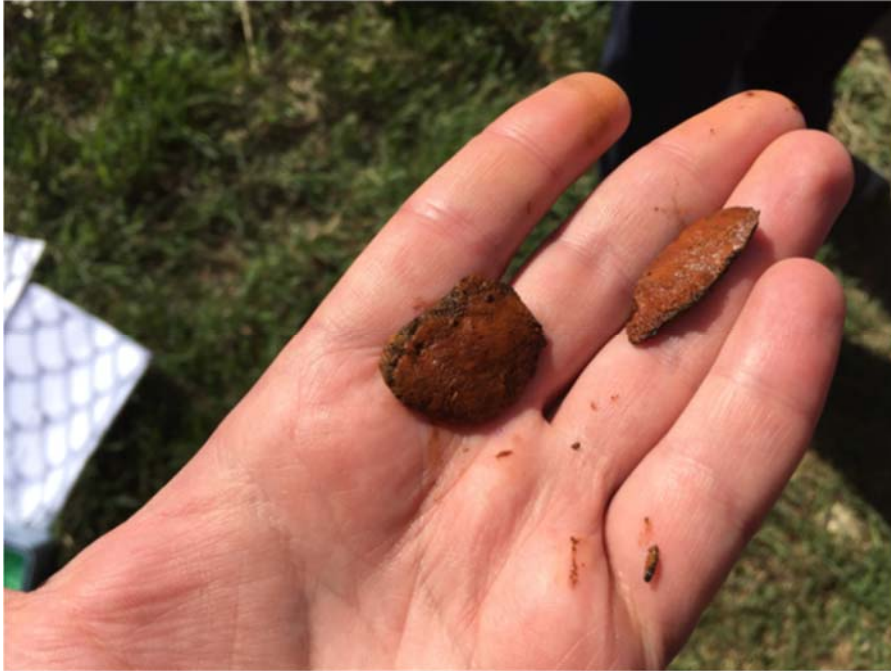
Figure 7. Tubercles removed on Loop #1 at 5 fps flushing velocity.
