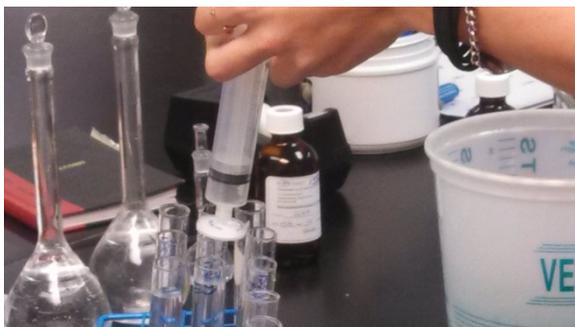
Samples for dissolved metals must be filtered using the filter specified in this method. The filter specified does not sorb or leach lead. The filter can be in a syringe, as in the picture here, or in a filter holder.
