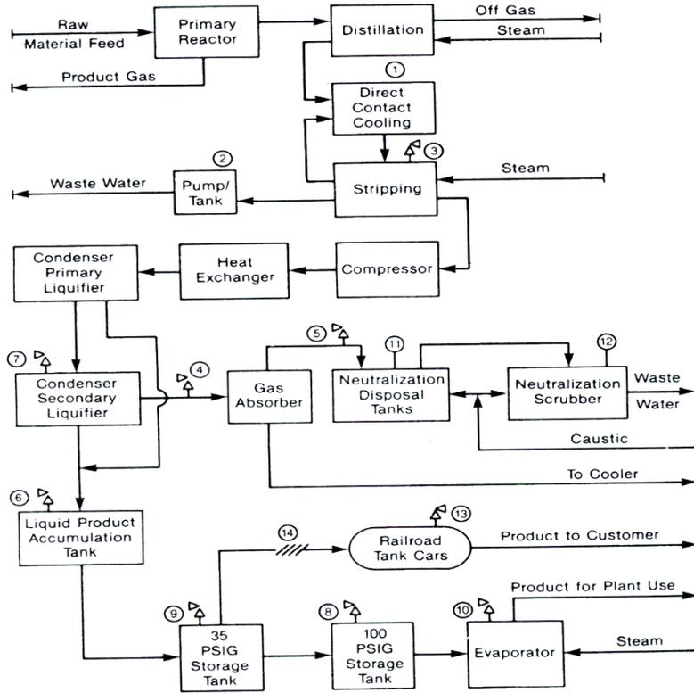
Illustration B – Example of a Process Flow Diagram
