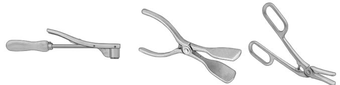
**Safe distance** is a form of operator protection that should be used only when other protection is not possible. Safe distance protection may be applied when the operator is not required to hold the work piece within 4-inches of the point of operation. Safe distance is measured 4-inches or more from tooling or the pinch point closest to the operator.
