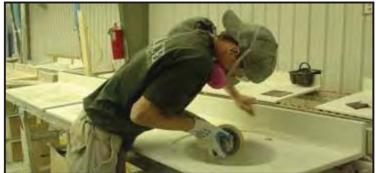
A worker using proper PPE during a sanding project
